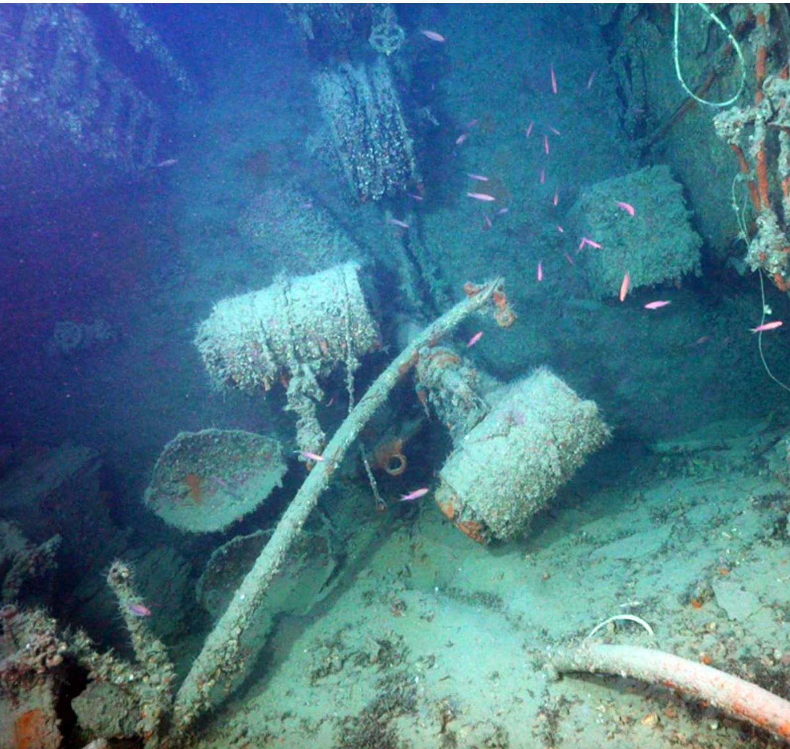
Photo: The portside two depth charges in their projectors. (photo: K. Hyttinen)
