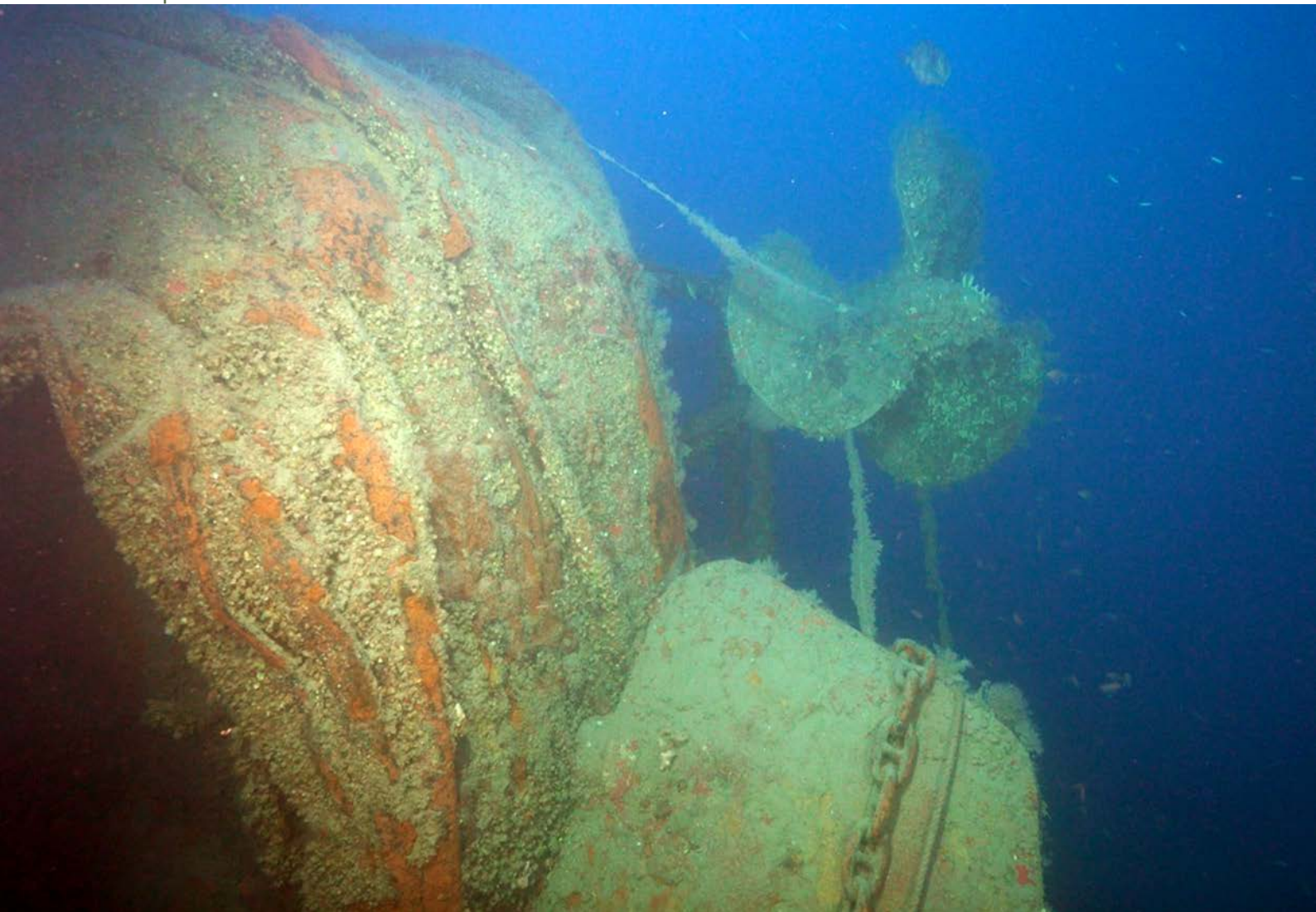
Photo: The characteristic impact buckles on the stern, the rudder and one of the propellers. (photo: K. Hyttinen)
