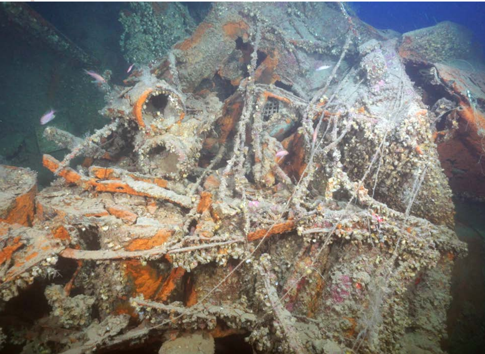
Photo: The stern of the ship and the twisted rails of the depth charge racks with the depth charges trapped inside. (photo: K. Hyttinen)
