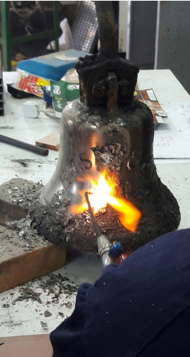
Photo: The heating method to remove the concretions outside the bell. (photo: Heritage Malta)
