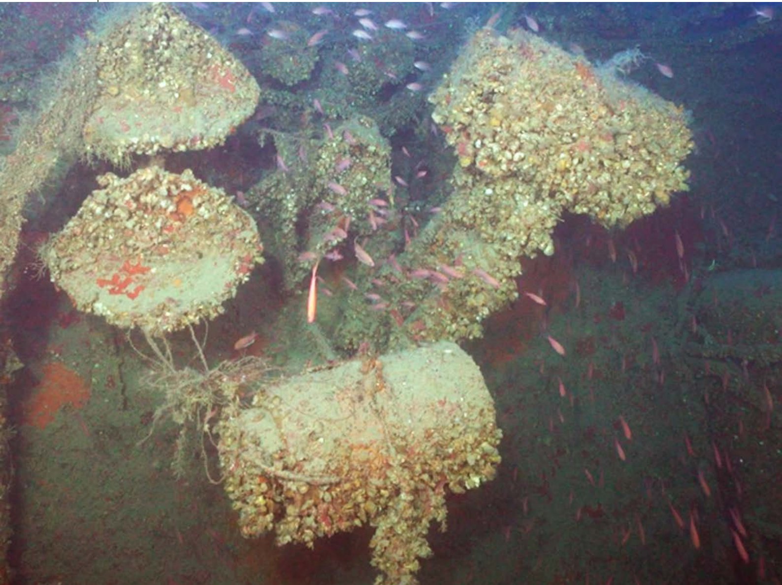
Photo: The starboard two depth charges in their projectors. (photo: K. Hyttinen)
