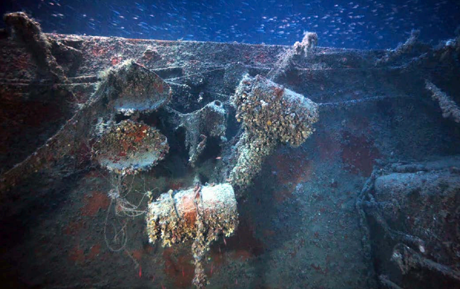
Photo: The starboard depth charges in their projectors. (photo: U-boat Malta Ltd.)
